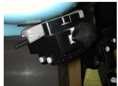
Figure 18. Head SAR Test Setup
