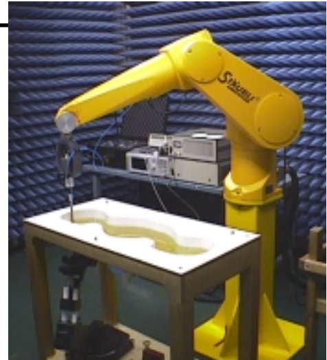
Fig1: The robot controlled probe during SAR measurement.
