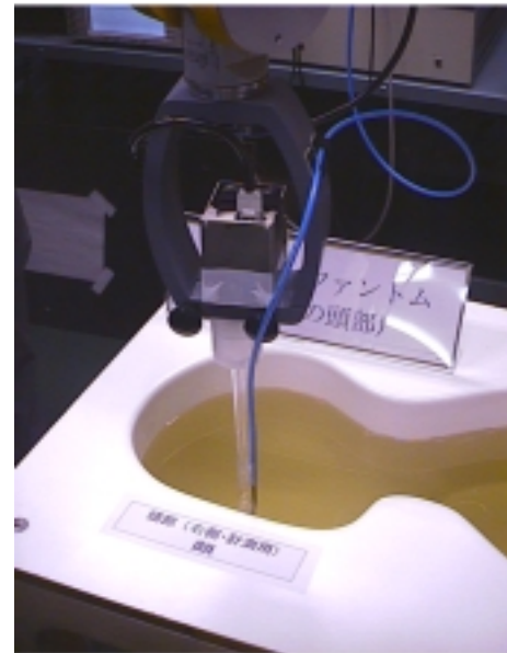
Fig2: The measurement set-up with a phantom containing tissue simulating liquid .
