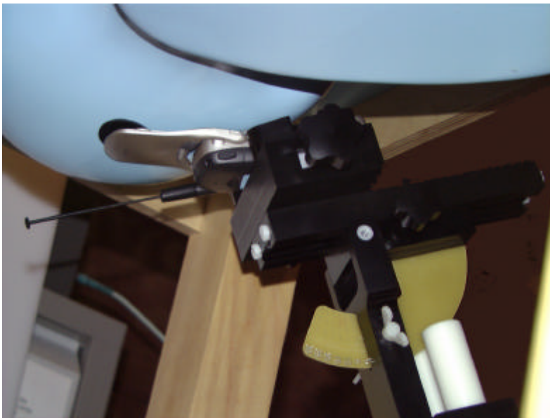
Fig 12. Sample of Handset Alignment with the Ear Canal of the Phantom
