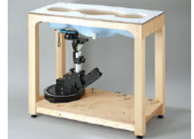
Fig. 8 Generic Twin Phantom
