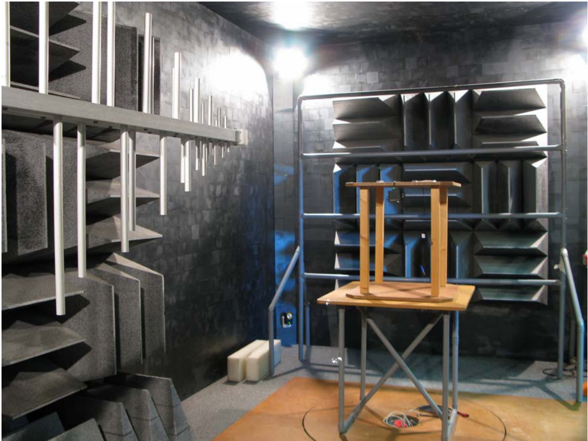
Photograph 1: radiated emissions test set up (0.03 - 1 GHz)
