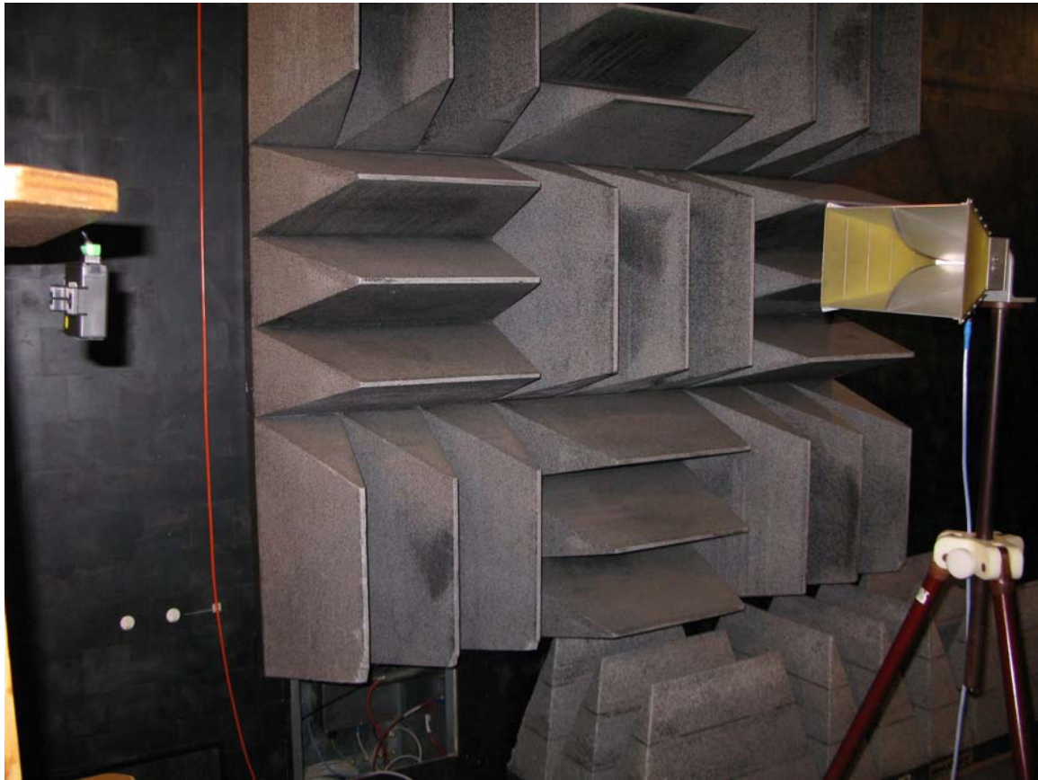
Photograph 2: radiated emissions test set up (1 - 18 GHz)
