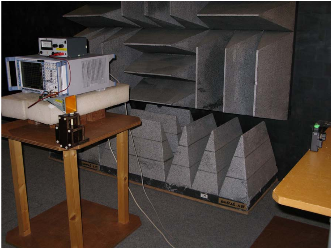
Photograph 4: radiated emissions test set up (26 - 40 GHz)
