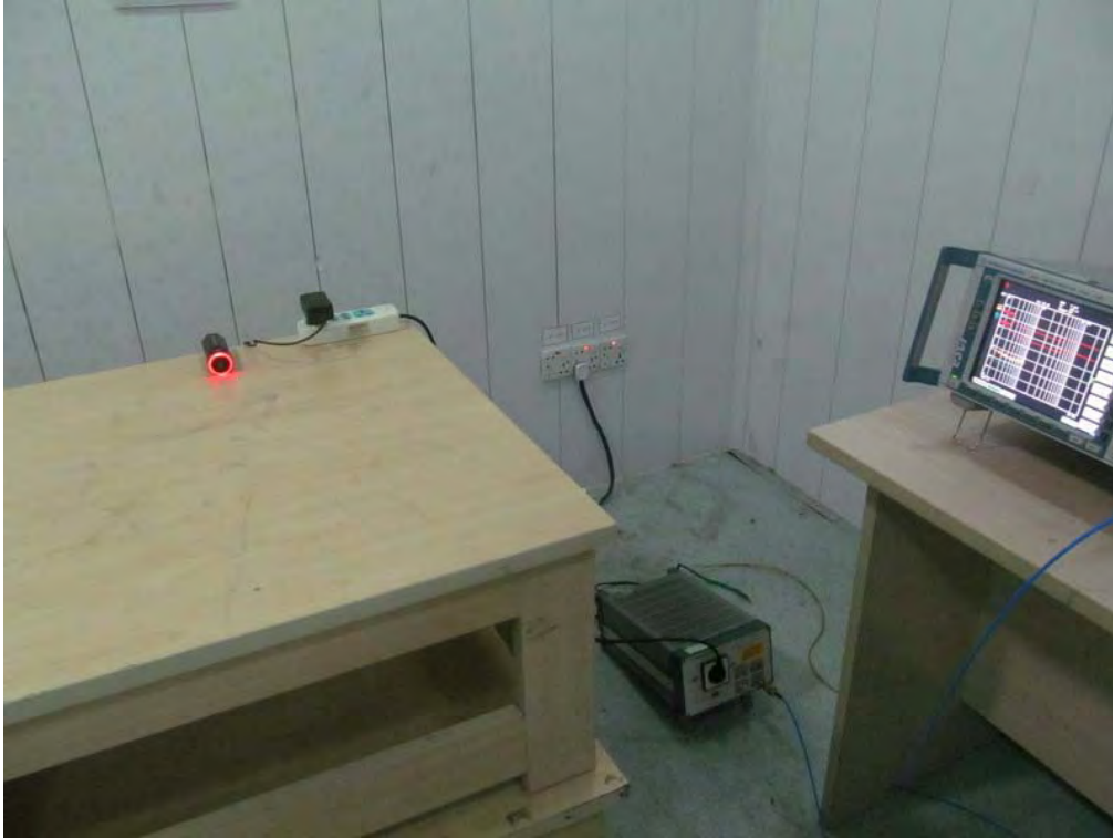
FCC RADIATED EMISSION TEST SETUP
