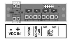
Figure: NFPA Dry Contact connection location inside the cabinet
