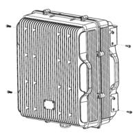
Figure: Secure the cabinet to the bracket
