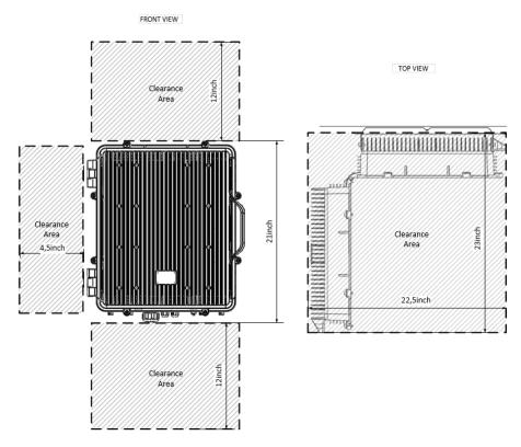
Figure: Mounting clearance WST012
