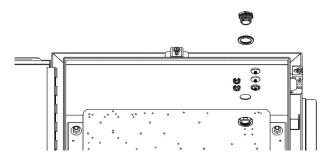
Figure: Install the sealing cup
