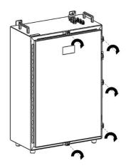
Figure: Secure Signal Booster cover
