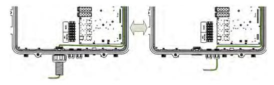
Figure: AC Routing through cable gland or conduit connector
