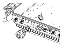
Figure: Remove the conduit connector
