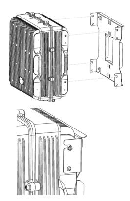
Figure: Hang the Signal Booster
