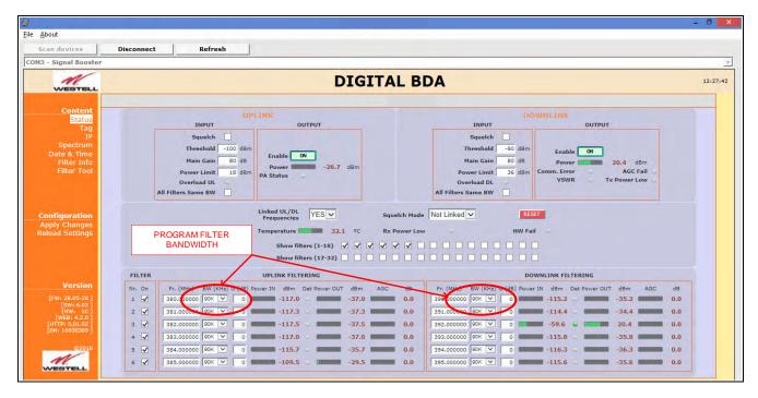
Filter bandwidth selection for narrow band filters version
