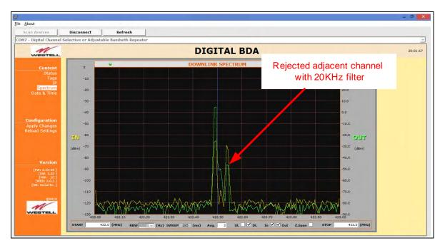
Adjacent channel rejection with 20KHz filter
