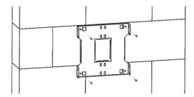
Figure: Bracket attachment to a wall using three fixing screws
