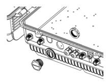
Figure: Install the sealing cup
