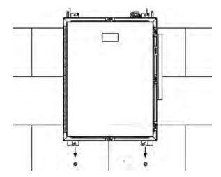
Figure: Hang the Signal Booster
