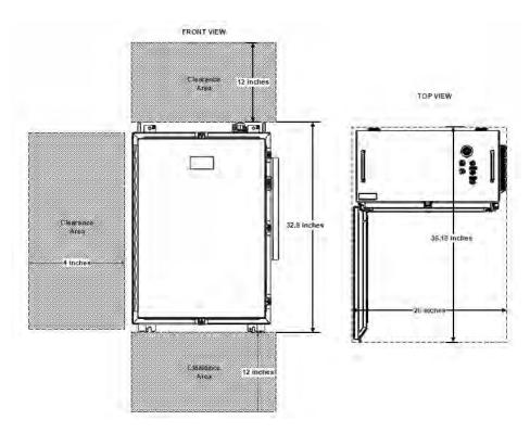
Figure: Mounting clearance WST021
