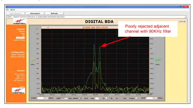
Adjacent channel rejection with 90KHz filter
