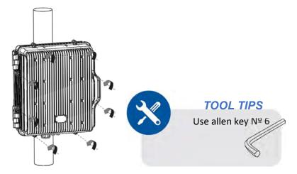
Figure: Release Signal Booster cover
