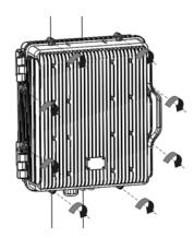
Figure: Secure Signal Booster
