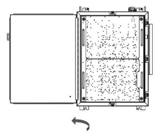
Figure: Open the Signal Booster cover
