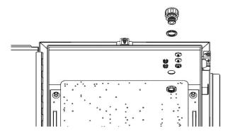
Figure: Remove the conduit connector
