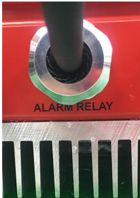
Figure 5-4: Alarm Relay 18-wire Gland Connector M6110
