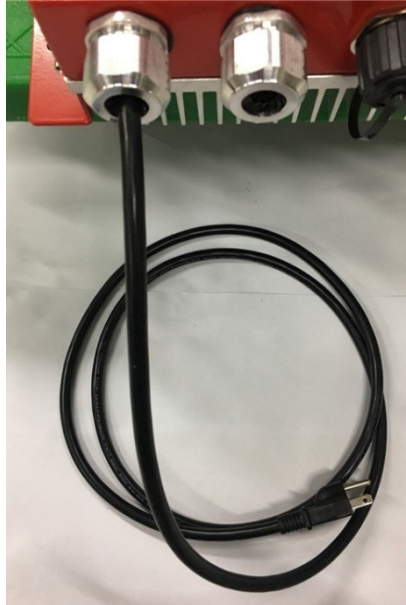
Figure 5-9: Power Cable Connected to Signal Booster
