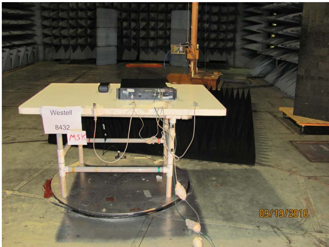
Photograph of Spurious Conducted Emissions Test Setup
