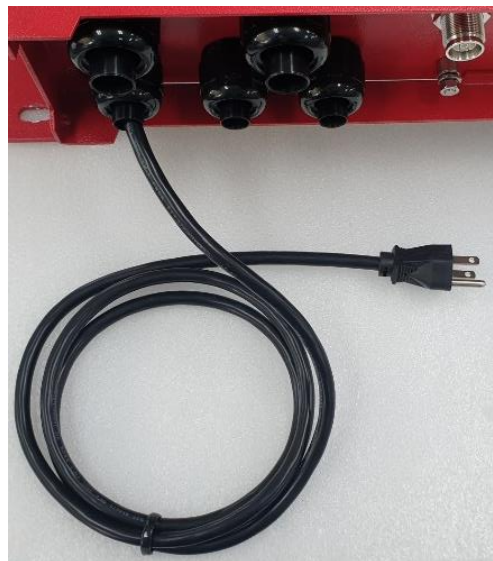
Figure 5-9: Power Cable Connected to Signal Booster
