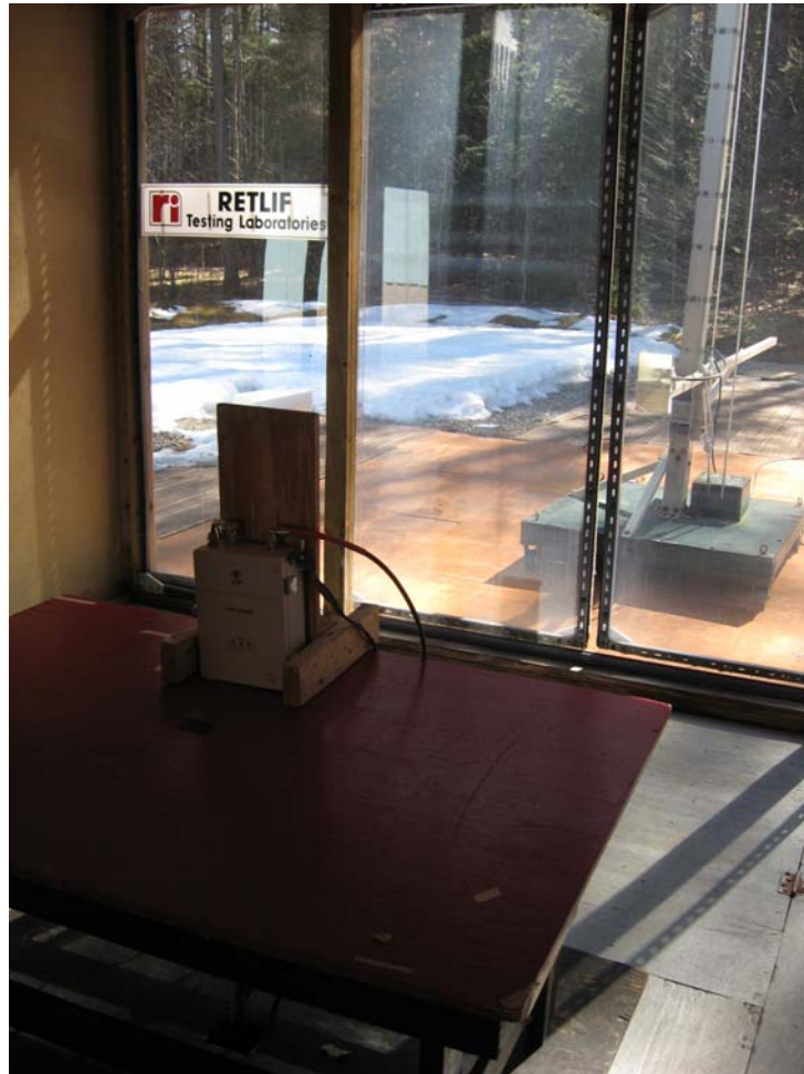
Test Setup, Horizontal Antenna Polarization
