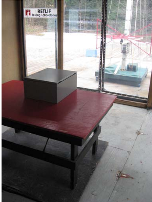
Test Setup, Horizontal Antenna Polarization
