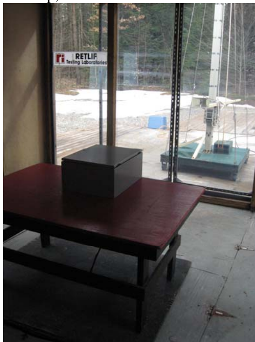
Test Setup, Vertical Antenna Polarization
