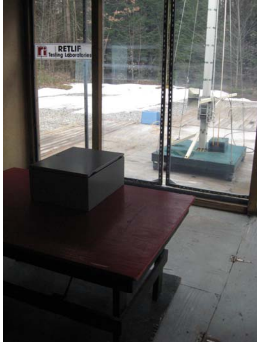
Test Setup, Horizontal Antenna Polarization
