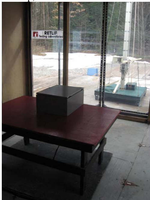
Test Setup, Vertical Antenna Polarization
