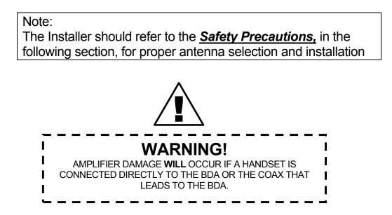
Important note: A high degree of isolation must be afforded to prevent any regenerative feedback in the system. Feedback of this nature causes the amplifier to emit a continuous signal of maximum amplitude and could, in some cases, interfere with normal operation of the cell site. The minimum required isolation of 70 dB can usually be obtained by mounting the outside antenna away from the edges of the roof. The use of window mounts or other non-rooftop mountings should be avoided.
