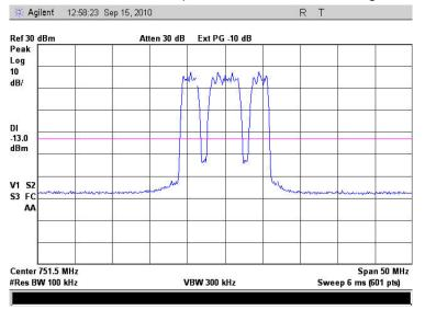
6.7.4. 781.5 MHz Inter-modulation products with W-CDMA Signal QPSK
