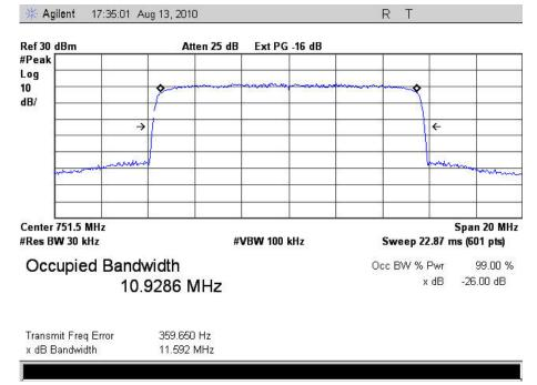
6.2.1.1. Occupied (99% Power) Bandwidth Measurement, 746-757 MHz
