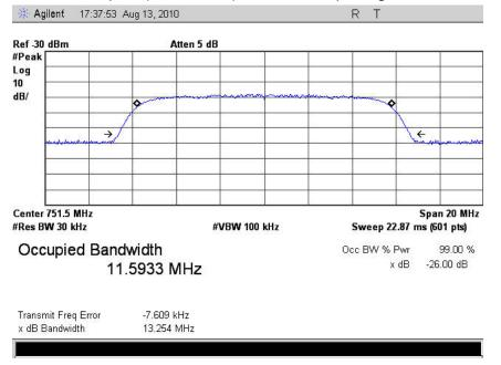
6.2.1.3. Occupied (99% Power) Bandwidth Measurement, 776-787 MHz
