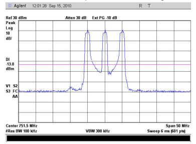
6.7.2. 781.5 MHz Inter-modulation products with CDMA Signal QPSK
