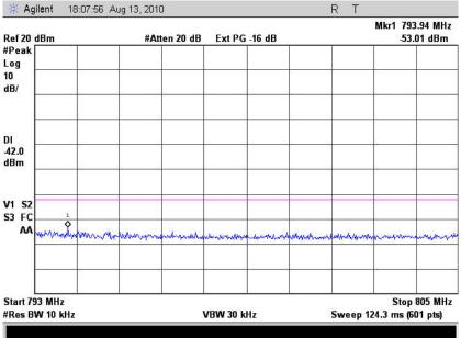
6.3.7. 746 MHz Bandedge Measurement using 9 MS/s 64QAM Signal
