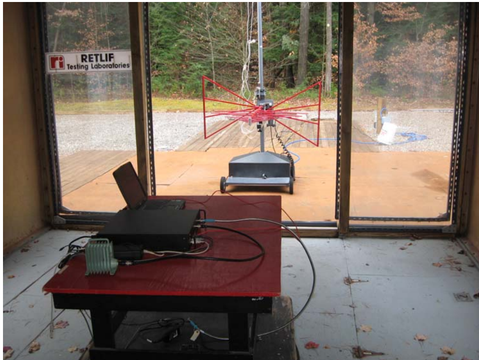
Horizontal Antenna Polarization
