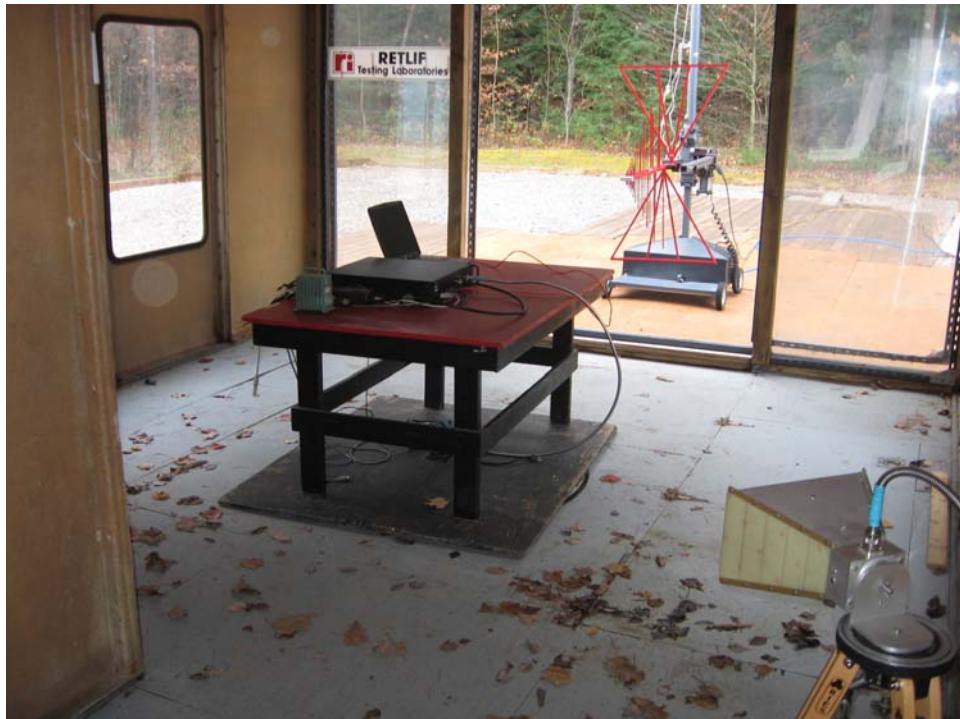
Vertical Antenna Polarization
