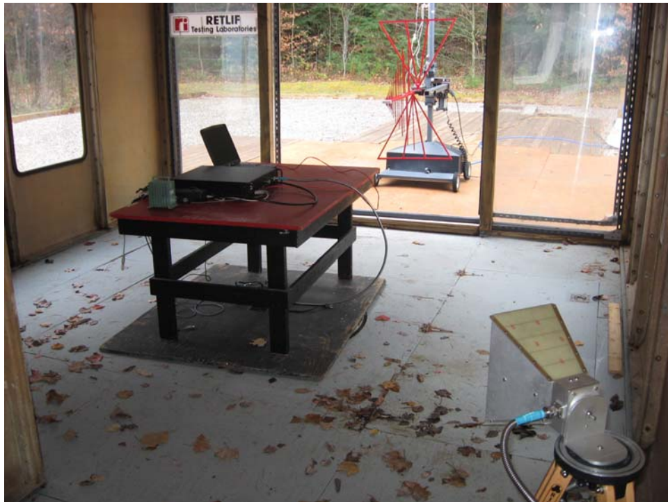
Horizontal Antenna Polarization
