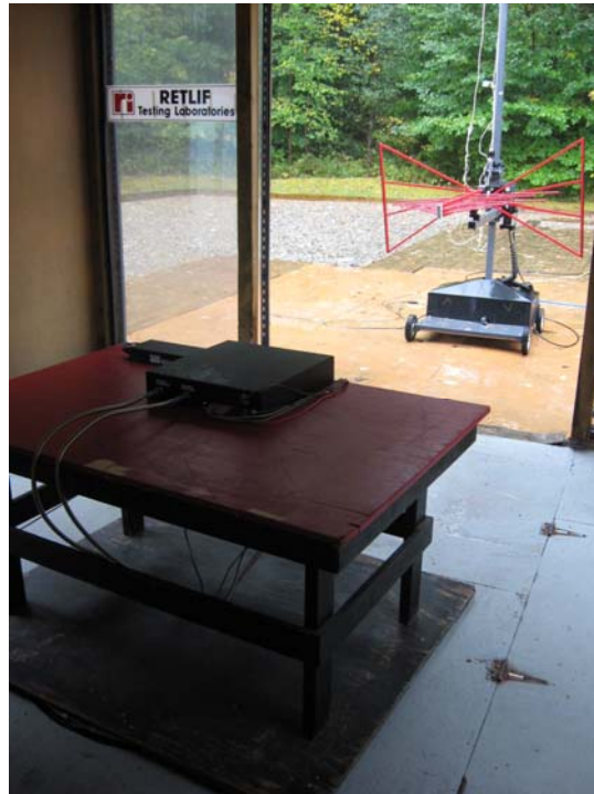
Horizontal Antenna Polarization
