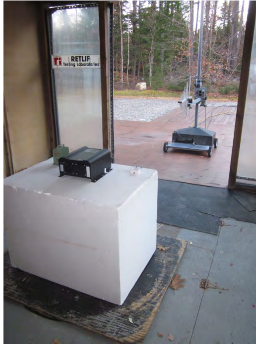
Spurious Emissions, Log Periodic, 200 MHz to 1 GHz, Vertical Polarization
