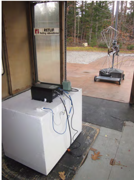
Spurious Emissions, Biconical, 30 MHz to 200 MHz, Vertical Polarization
