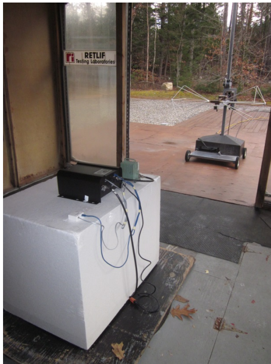
Spurious Emissions, Biconical, 30 MHz to 200 MHz, Horizontal Polarization
