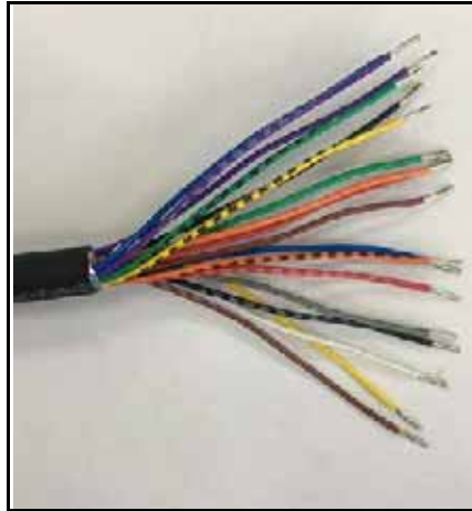
Figure 4-6 Stripped alarm wire
