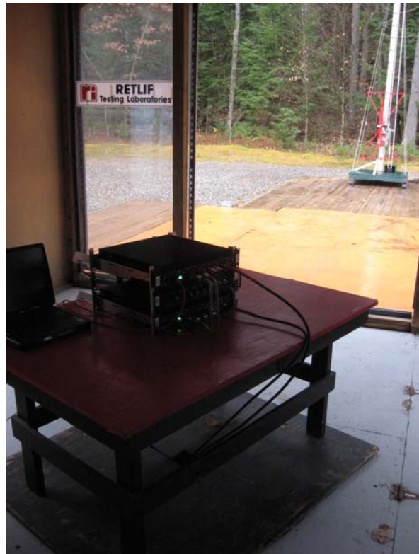
Vertical Antenna Polarization, 30 to 1000 MHz
