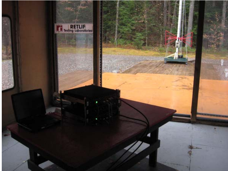
Horizontal Antenna Polarization, 30 to 1000 MHz
