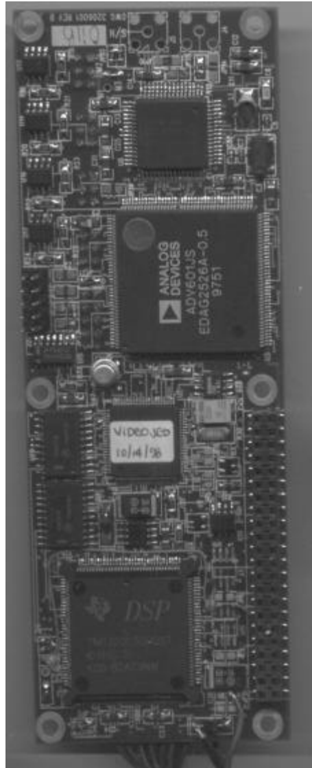
RFU pcb DSP uP Rev. B #011B component side
