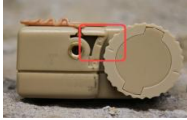
Figure 3-5: Battery Switch Cover Rotated to ON Position
