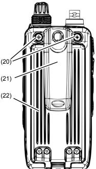
All rubber covers must be closed and the battery pack installed for the receiver to be waterproof (IPX5).
