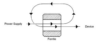
The ferrite must be installed as near as possible to the device!
