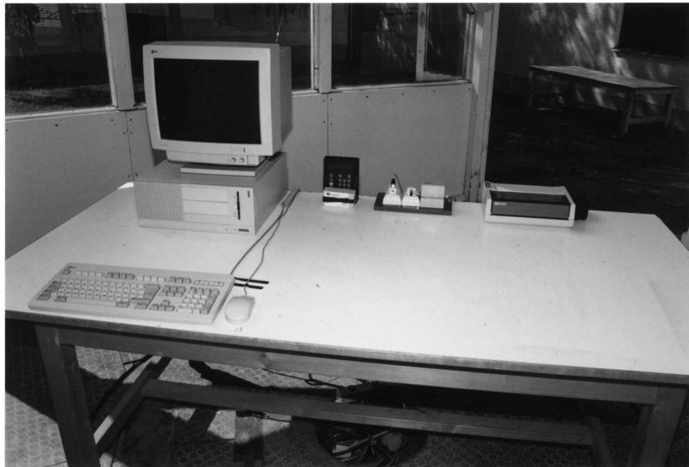
Test setup radiated emission test 30 MHz - 1000 MHz
