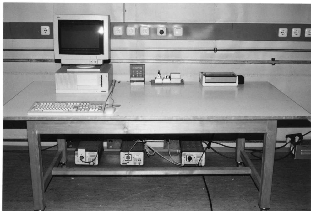
Test setup conducted emission test 450 kHz - 30 MHz
