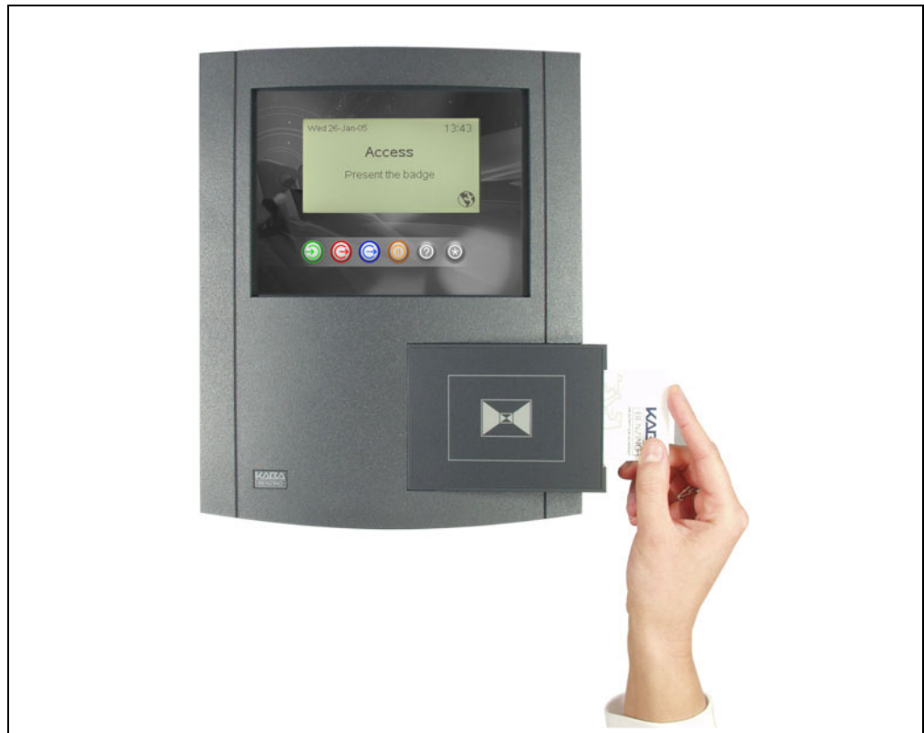
Fig. 59: Insert inductive badges
