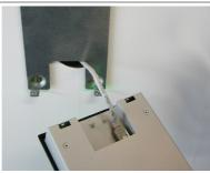
For PoE devices just plug in the Ethernet cable. Note that the device will be started immediately if you have already connected the other end into the switch.
