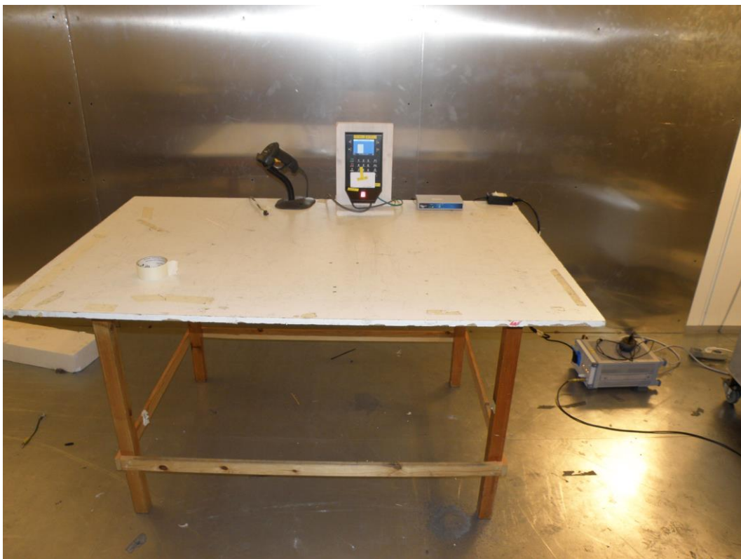
Photograph 4, AC mains conducted emissions test, configuration 2
