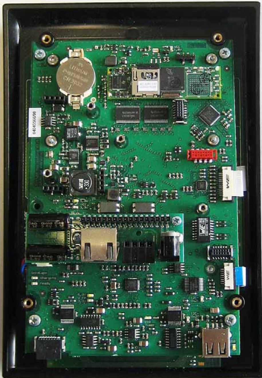
TT1100 front-panel, rear-view, with Mainboard. -> PoE module removed -> RFID module removed -> Reader carr. removed
