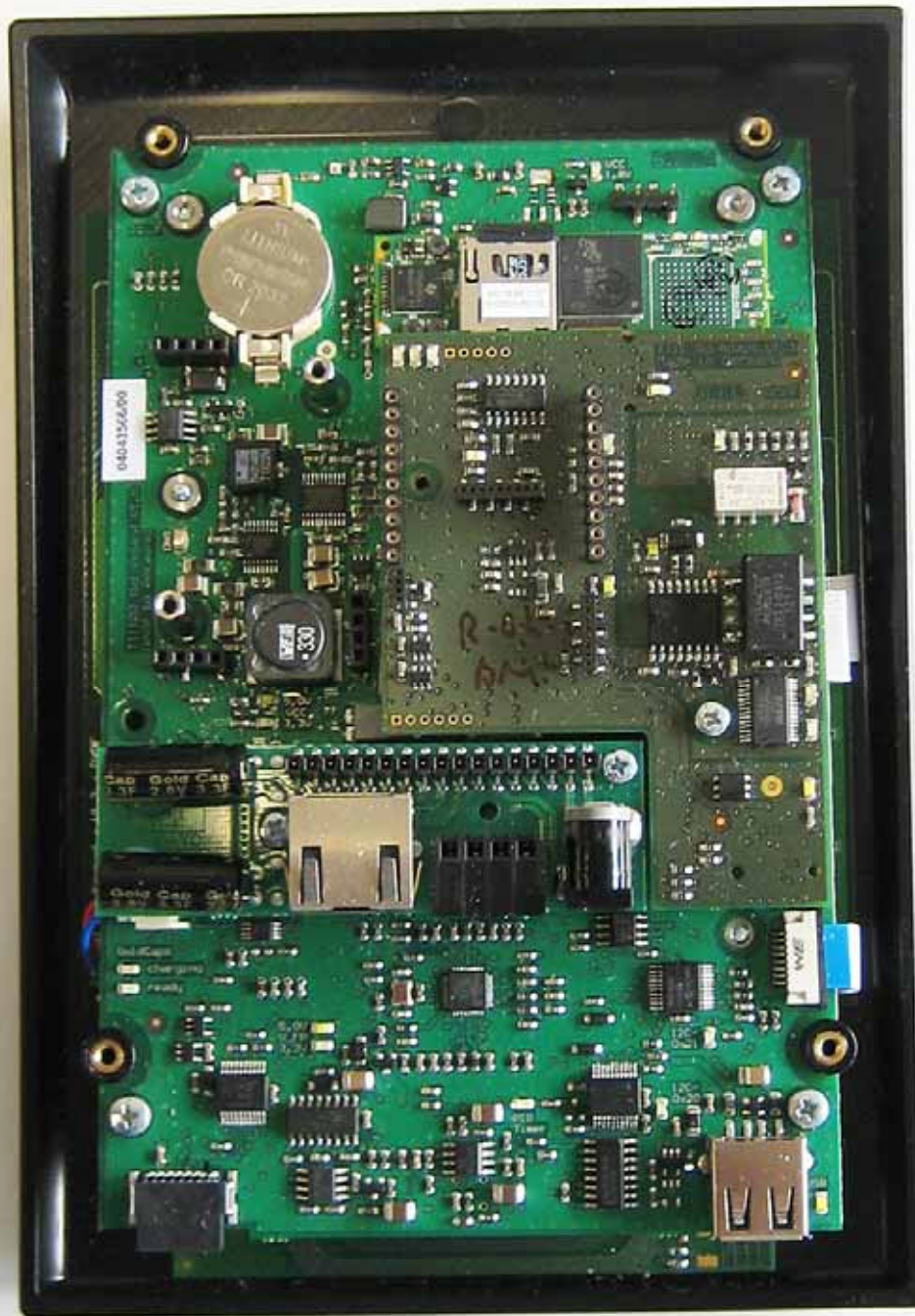
TT1100 front-panel, rear-view, with Mainboard. -> PoE module removed -> RFID module removed
