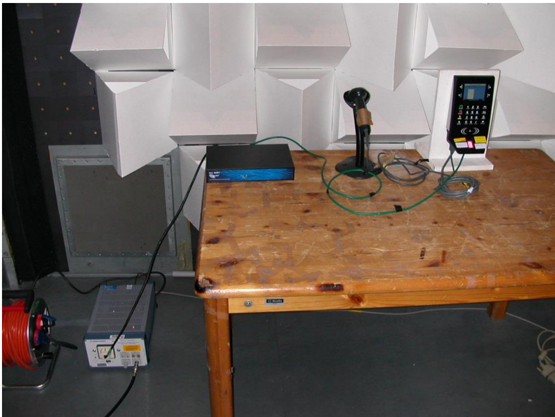
Figure 4 EUT / test set up - spurious conducted emissions
