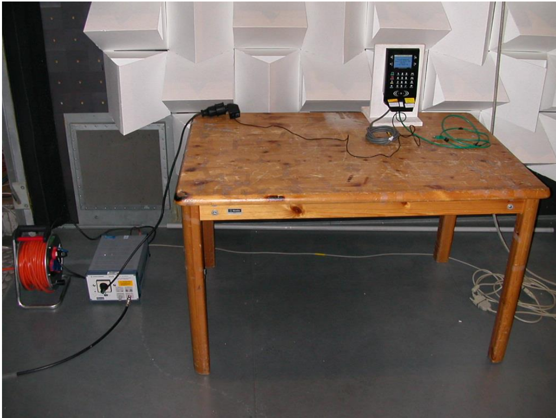
Figure 3 EUT / test set up - spurious conducted emissions
