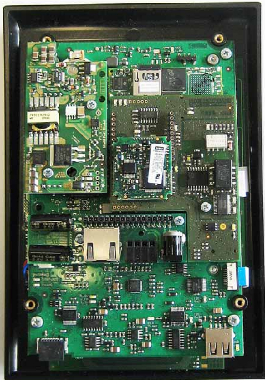
TT1100 front-panel, rear-view with Mainboard and all modules mounted
