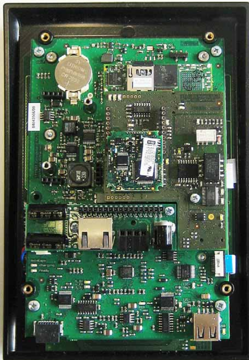
TT1100 front-panel, rear-view, with Mainboard. -> PoE module removed
