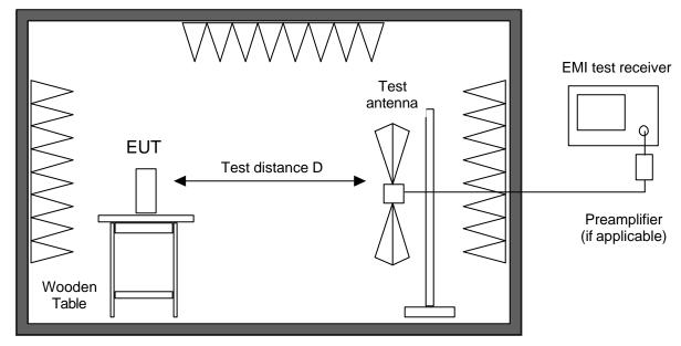
Alternate test site (semi anechoic room)
