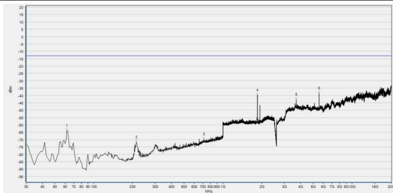
(Plot J1: HSUPA 1900MHz Channel = 9262, Test Antenna Horizontal)
