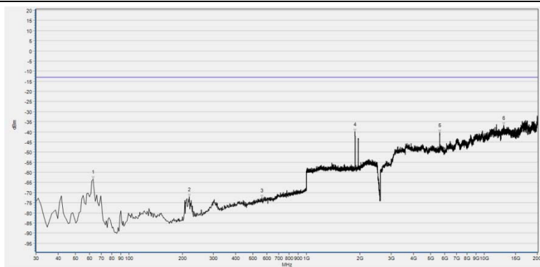
(Plot L3: HSPA+ 1900MHz Channel = 9400, Test Antenna Horizontal)
