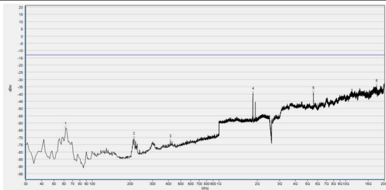
(Plot H1: HSDPA 1900MHz Channel = 9262, Test Antenna Horizontal)
