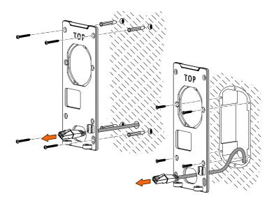
The mounting plate may not be mounted twisted. The screws may only be tightened slightly. The mounting plate may not be deformed or bent.
