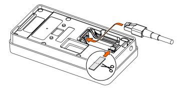
3. Insert the seal with suitable cable passage (see table) into the sealing cap.
