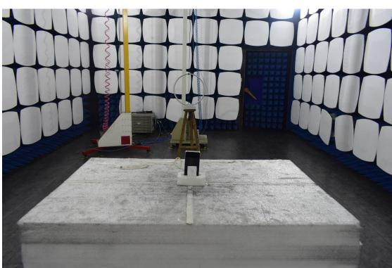
3. Radiated emission (9KHz-30MHz)
