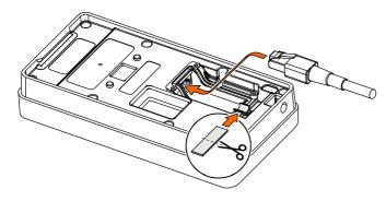
3. Insert the seal with suitable cable passage (see table) into the sealing cap.
