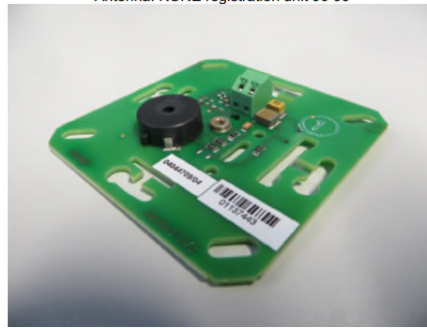
Antenna: KONE registration unit 90 00
