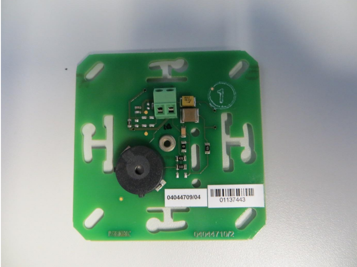
Antenna: KONE registration unit 90 00
