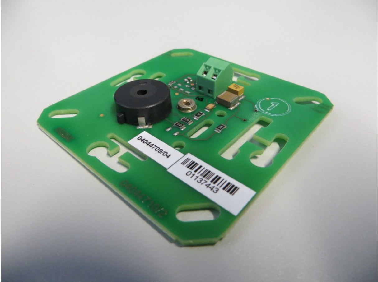
Antenna: KONE registration unit 90 00
