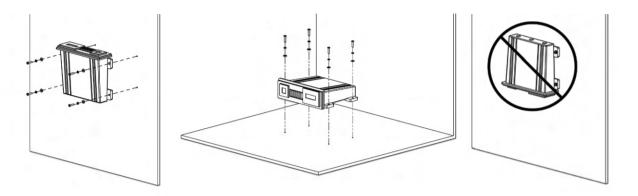
The in.stream system should be installed on an even horizontal or vertical surface.
