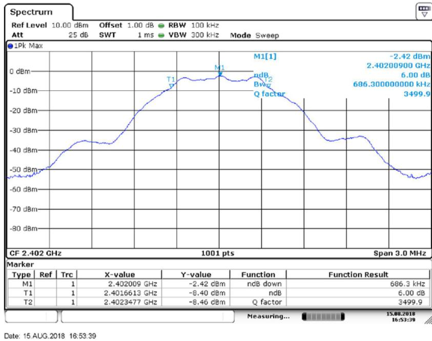
Test Model DTS (6dB) Bandwidth
