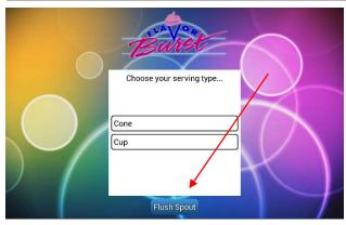
NOTE: IT IS NOT RECOMMENDED THE "FLUSH SPOUT" BUTTON BE ACTIVATED IN SELF-SERVE ENVIRONMENTS. THOSE NOT FAMILIAR WITH THE EQUIPMENT MAY ACCIDENTLY ACTIVATE THE FLUSHING FUNCTION WITHOUT REALIZING WHAT IT DOES OR HAVE A CONTAINER TO CATCH THE SANITIZER SOLUTION.
