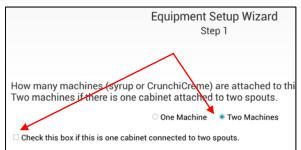
If you have two Flavor Burst cabinets operating from one Touch Panel (i.e. if there is a Base unit attached to the main Flavor Burst system), you will need to tell the system if they are both connected to the same spout (model Base-1S) or separate spouts (Base-2S).
