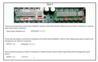
If two cabinets are attached, the system needs to know which ports are being used for each cabinet and spout. Follow the cables from each cabinet to the electronics board to determine which cabinet is connected to which ports.
