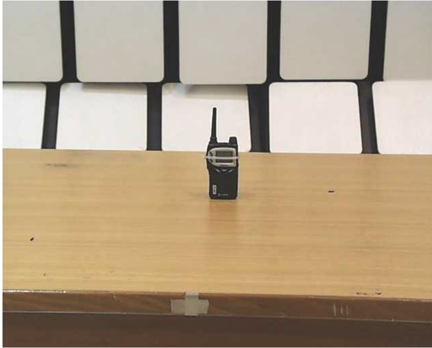
Effective Radiated Power Test Setup Close-up View
