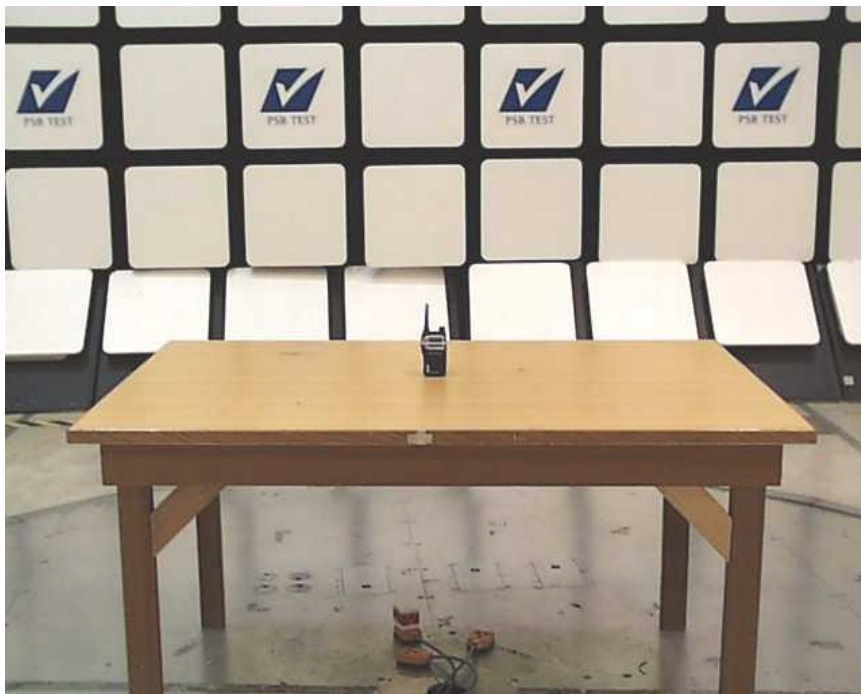
Effective Radiated Power Test Setup General View
