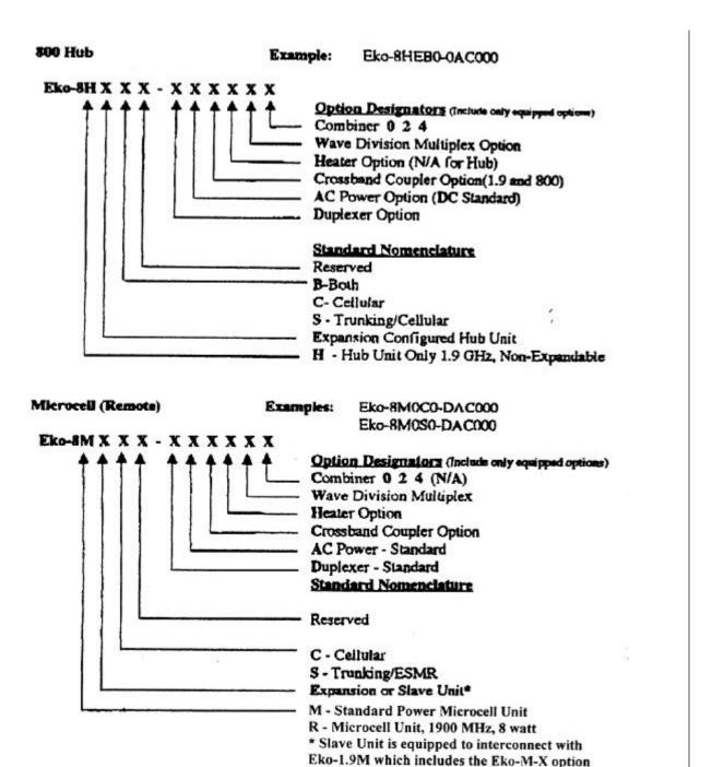
For the 1900 MHz unit, the 8 shown in these descriptions is replaced by 1.9
