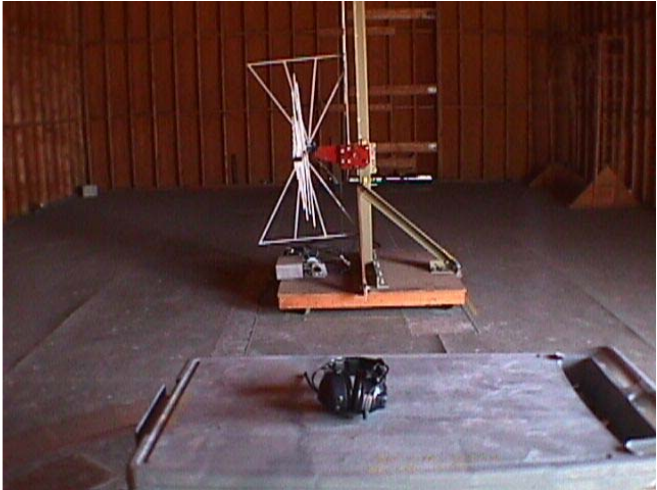
Radiated Emissions at 3 Meters Distance Orthogonal Position # 1
