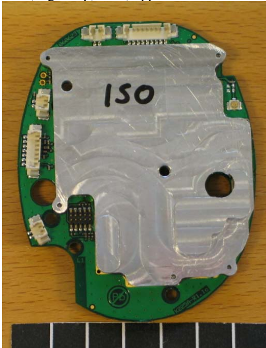
EUT, right cap, PCB, upper side, outer shield dismantled
