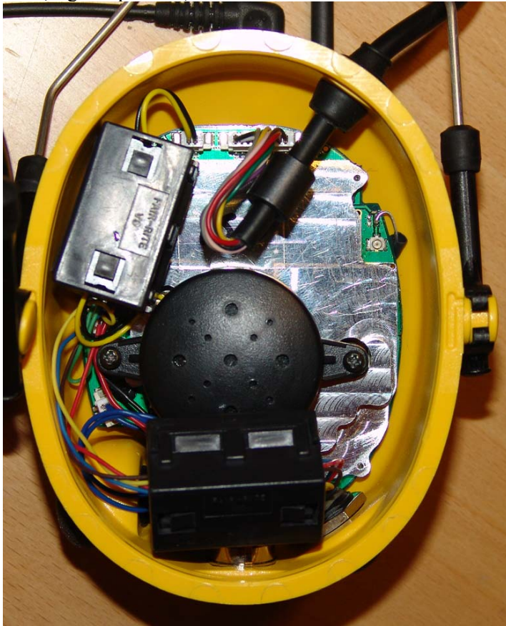
EUT, right cap inside, close-up (speaker dismantled)
