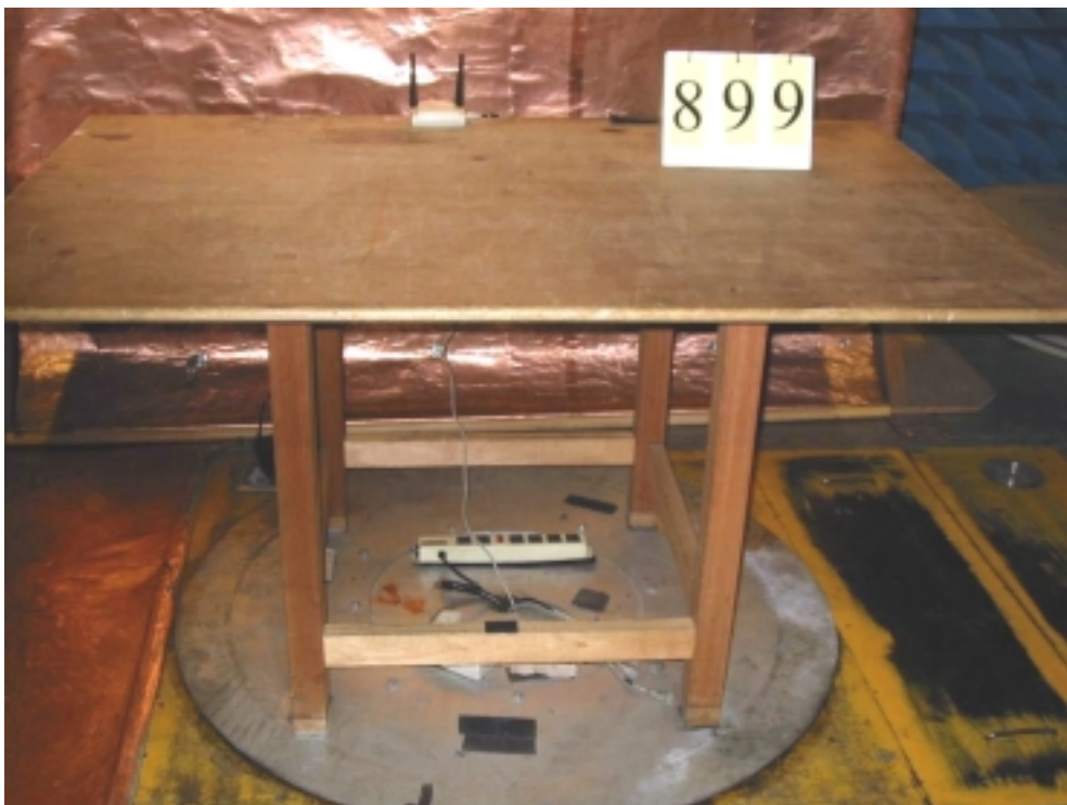
Conducted Emissions Test Placement
