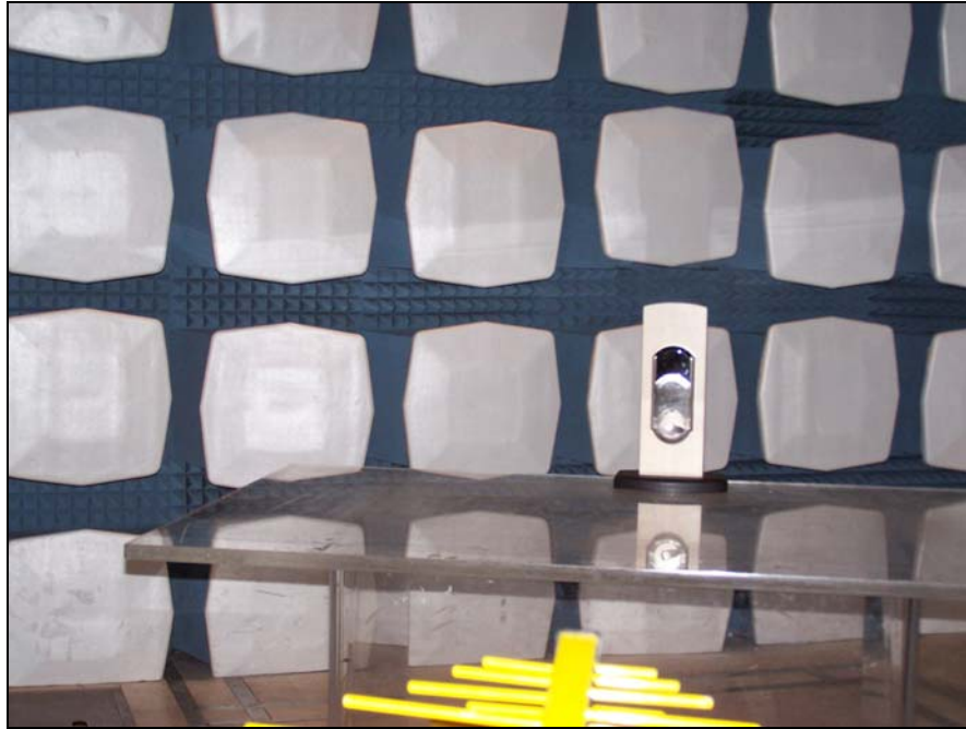
Photograph 4. Radiated Test Setup, Below 1 GHz
