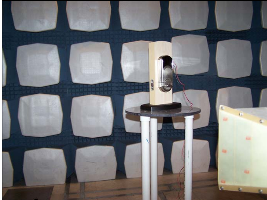
Photograph 3. Radiated Test Setup, Above 1 GHz
