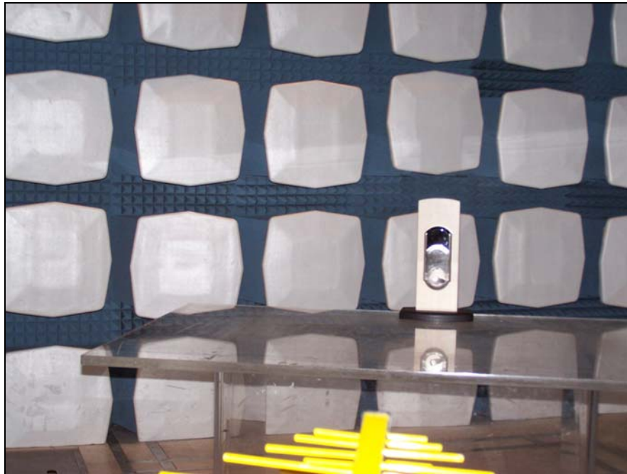
Photograph 2. Radiated Test Setup, Below 1 GHz
