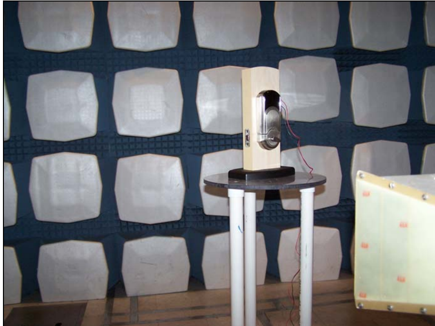
Photograph 5. Radiated Test Setup, Above 1 GHz
