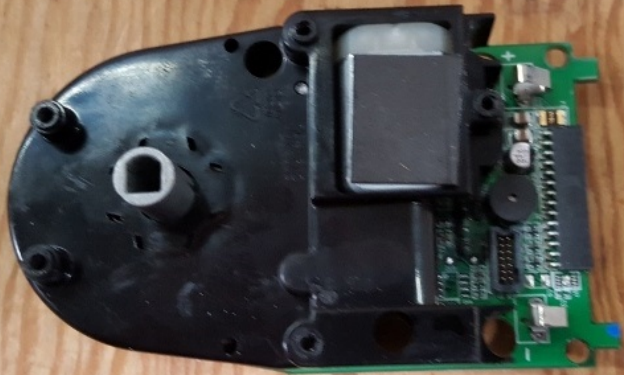
Internal Photos: Internal Lock
